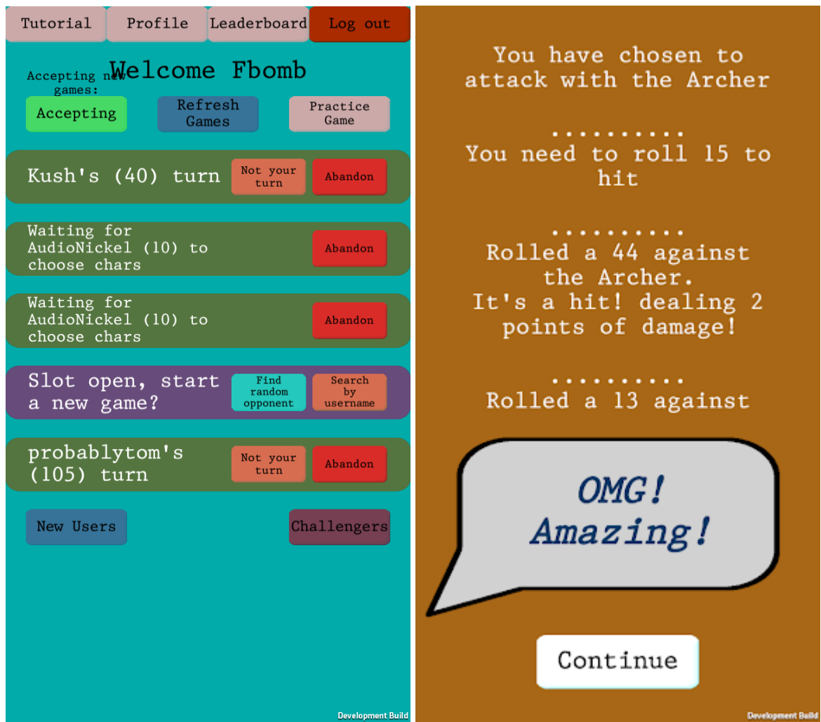
Figure 5.3: UI bugs raised in closed testing. Overlapping text and a player's skill not showing (decile and the player not being shown who they have attacked (right)).
